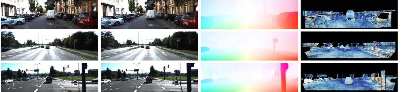
Fig. 4. Qualitative results of our pretrained model on training pairs of KITTI Flow 2015 dataset. From left to right: input image of first frame, input image of second image, colorized flow prediction, error map. The error map is drawn by development kits provided by KITTI dataset, where the blue regions represent correct predictions and the red areas indicate incorrect estimates.
