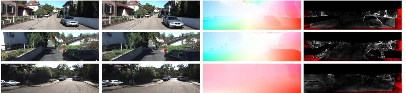
Fig. 5. Qualitative results of our final fine-tuned model on testing pairs of KITTI Flow 2012 dataset. From left to right: input image of first frame, input image of second image, colorized flow prediction, error map. The error map is captured from our submission, which scales linearly between 0 (black) and  $\geq 5$  (white) pixels error. Red denotes all occluded pixels, falling outside the image boundaries.
